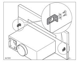
When fitting an 80 cm or a 90 cm appliance into a 60 cm unit, unscrew the brackets on the deflector plate whilst it is pulled out.
